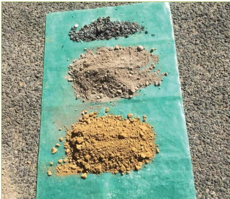
Figure 2.2.12 – BH4: Existing Pavement Materials (Top to Bottom)
