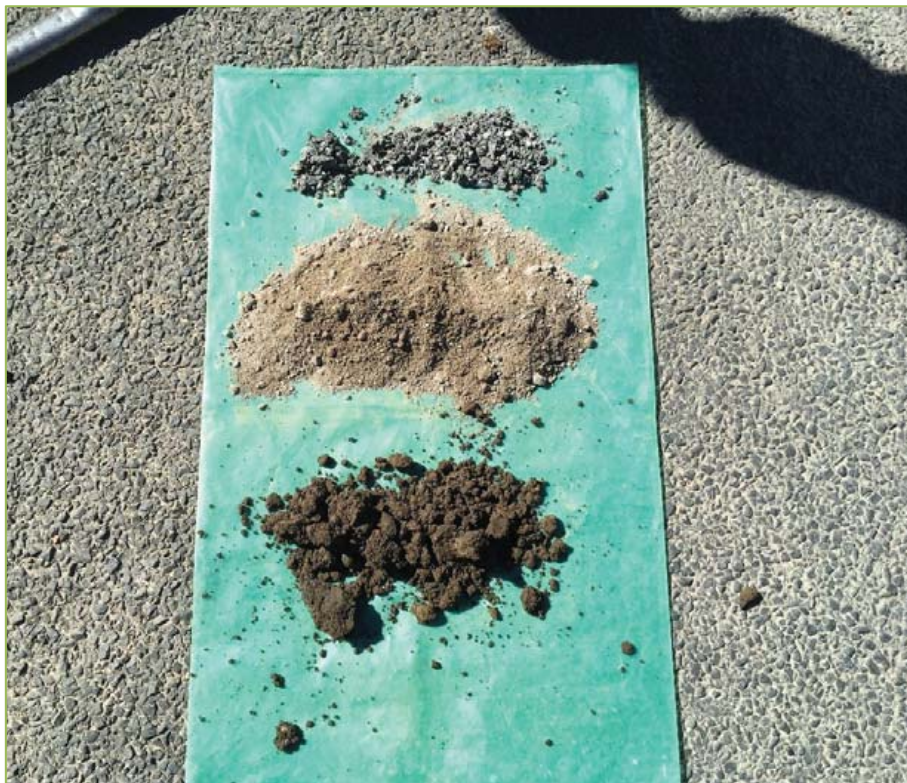
Figure 2.2.6 – BH3: Existing Pavement Materials (Top to Bottom)
