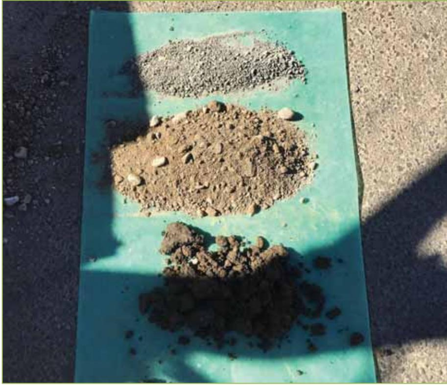
Figure 2.2.3 – BH1: Existing Pavement Materials (Top to Bottom)
