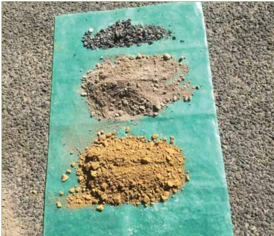
Figure 2.2.12 – BH4: Existing Pavement Materials (Top to Bottom)
