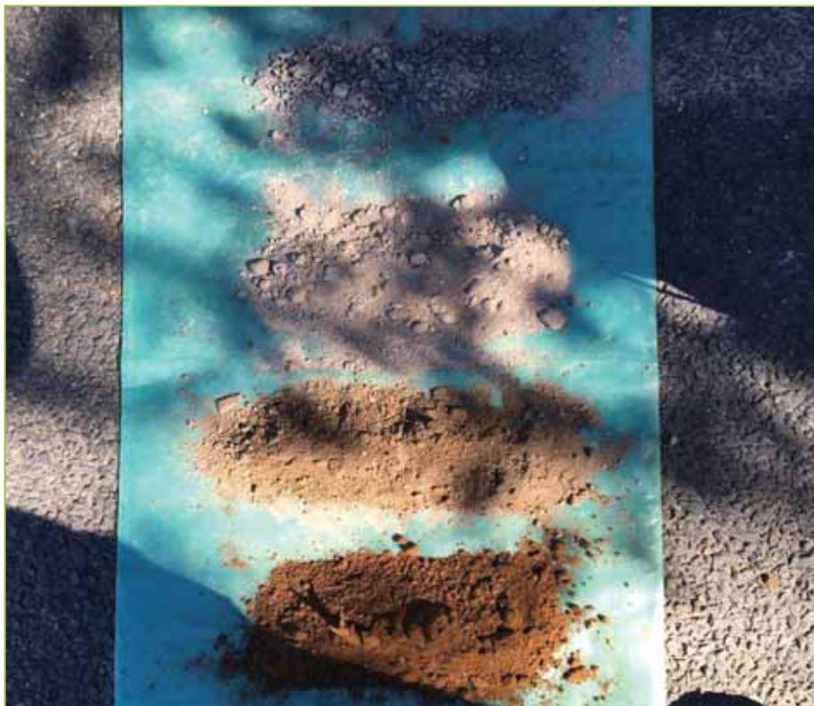
Figure 2.2.15 – BH5: Existing Pavement Materials (Top to Bottom)
