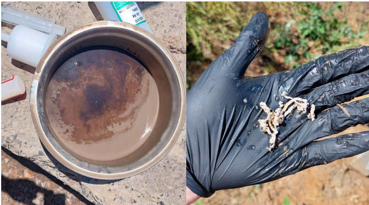
Left: Oily sheen on well water removed from BSM2, possibly related to fluid utilised in drilling of new bore.
